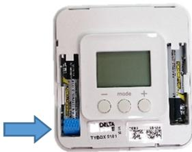
3. Remove the block cover back to the receptor
