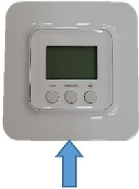
2. Remove the battery power storage protection
